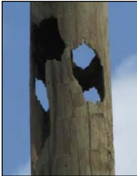
Figure 9-21. Woodpecker nesting cavity resulting in a virtually hollow pole.
