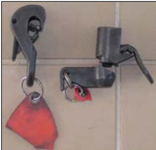
Figure 8-19. Flapper-type markers with deteriorated plates.
