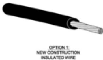
Figure 7-6. Insulated (covered) jumper wire for new installations.
