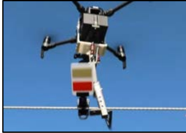
Figure 8-8. Drone-based line marking.
