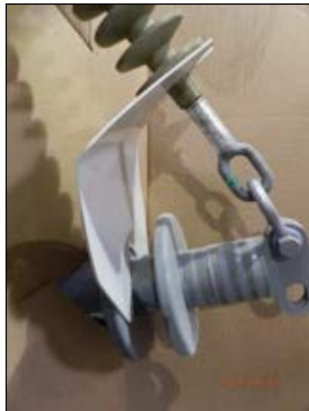
Figure 6-8. Kaddas Enterprises, Inc. prototype horizontal line post shield guards against contact with the energized portion of a braced post insulator.
