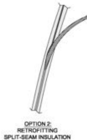
Figure 7-7. Insulated (covered) jumper wire for retrofitting.
