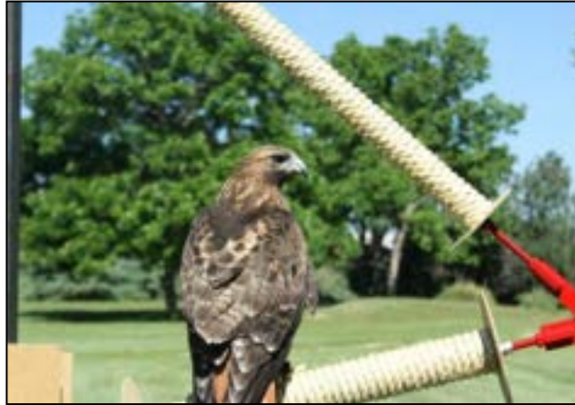
Figure 6-7. Mock 69kV braced post insulator configuration with a Red-tailed Hawk.
