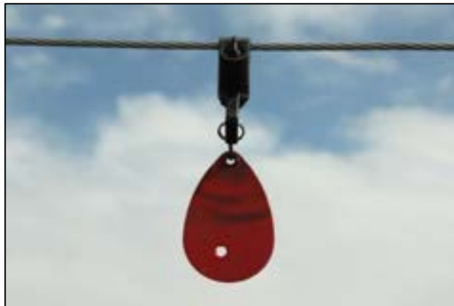
Figure 8-18. Flapper-type marker with a bullet hole.
