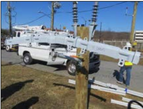
Figure 5-14. Hendrix Molded Products conductor cover.
