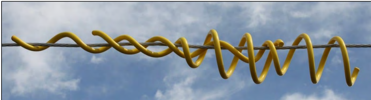
Figure 8-25. Improperly installed markers that have shifted.
