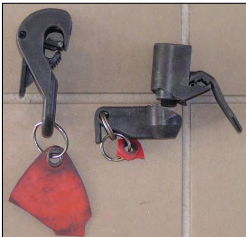
Figure 8-19. Flapper-type markers with deteriorated plates.
