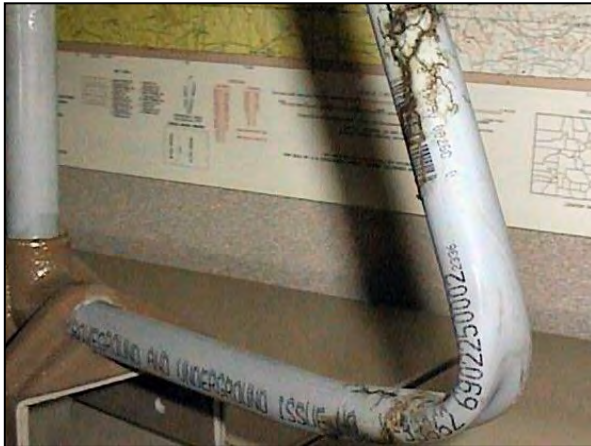
Figure 5-108. Flash marks on discourager.
