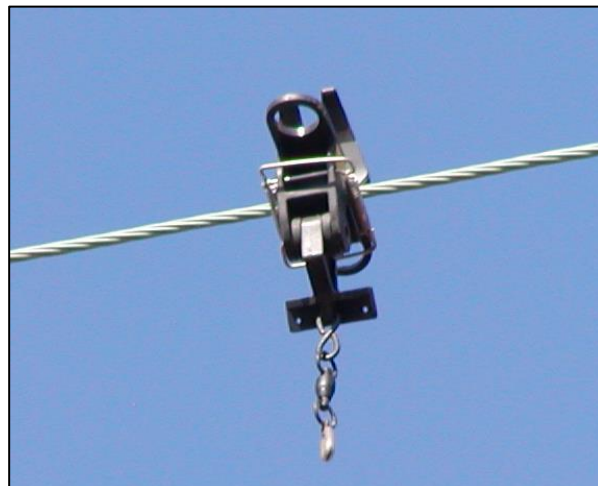
Figure 8-20. Broken hardware on active line marker
