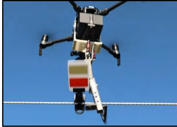
Figure 8-8. Drone-based line marking.
