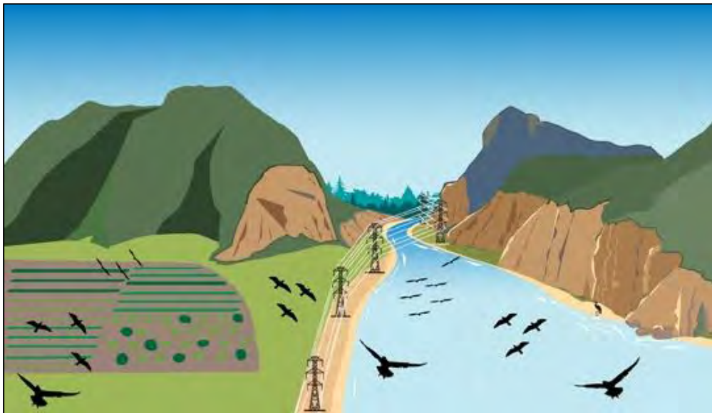
Figure 2-20. Topography can concentrate birds in potentially hazardous flight corridors.
