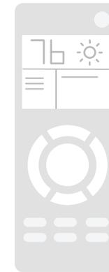
Avoid frequent adjustments to the temperature setting. Your ductless heat pump is designed to adjust to changing conditions automatically and efficiently. Note that heat pumps do take a little time to adjust to new settings, so remember to be patient when making adjustments. If you do prefer to lower the temperature at night or when you leave home, a change of no more than 3° is recommended.
